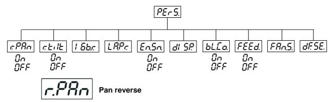
This function allows you to invert the pan movement. Use the **[Up]** and **[Down]** buttons to select **"On"** if you wish this feature or **"Off"** if you don't wish this feature and press **[Enter]** to confirm or **[Mode]** to cancel and return to the menu.
