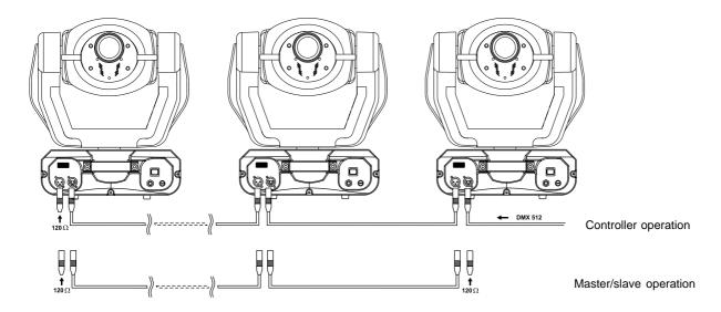
Only use a stereo shielded cable and 3-pin XLR-plugs and connectors in order to connect the controller with the fixture or one fixture with another.
