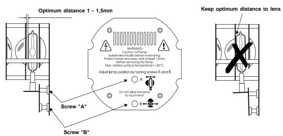
The SPOT 250 XT lampholder is aligned at the factory. Due to differences between lamps, fine adjustment may improve light performance.
